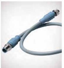
Double-ended cordsets are used for trunk or drop lines and make for a secure connection and simple timesaving installation. The connectors are keyed for error-free connection and they are waterproof for continued operation even while submerged in the bilge.
