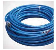
This 25 meter length Mid size cable with a Micro female connector on one end is intended for installation of devices such as Maretron's WSO100 Weather Station. The female connector should point towards the device and a field attachable male connector should be made onto the end connecting to the rest of the backbone.
